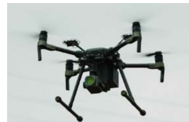
Dajiang M210 Load:X5S high-resolution visible light camera
