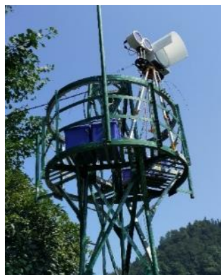
Large aperture scintillation(1) and microwave scintillation(1) 大孔径闪烁仪(1)和微波闪烁仪(1)
