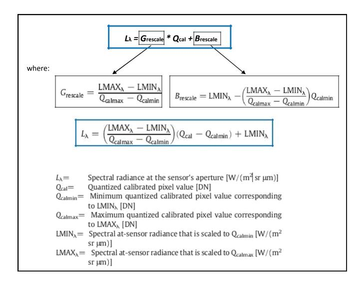
The LMIN and LMAX values are the spectral radiances for each band at digital numbers 1 and 255, respectively. One set exists for each gain state (i.e., high and low gain). The low-gain setting is used for bright surfaces (higher dynamic range with low sensitivity) and the high-gain is used for darker surfaces (lower dynamic range but higher sensitivity). The variables needed for the equation above can be found in the tables below.
